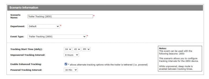
Note that live locates are unavailable in sleep mode, but the Trailer Tracking (2850) scenario will continue to operate, sending locates on the configured schedule. Tracking may be enabled at a frequency of up to 3 locates per day, every 8 hours from the start time set by the user. To preserve battery life, the interval may be set to 12 hours (2 locates per day), or once every 24 hours.
