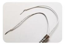
The sensor can be installed anywhere around the door to be monitored, so that the two halves are in close proximity (within 1 cm) when the door is closed. Once connected to the beacon, the events are generated when the two halves of the sensor are separated (for a Door Opened event) or when they come in close proximity (Door Closed).
