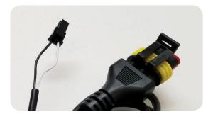
The 1-Wire Data connection on the 2840 wiring harness is wire 9 (White/Blue).
