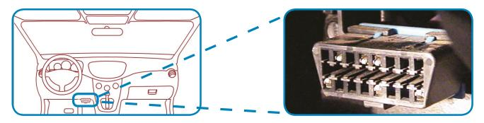
With the vehicle ignition turned off, install the beacon by pressing it firmly onto the vehicle port. The beacon is powered from the vehicle battery, allowing communication to start right away. Connectivity can be confirmed by looking at the LEDs (see LED Indicators below) and by checking the portal for ignition events once the vehicle is started.
