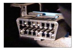
With the vehicle ignition turned off, install the beacon by pressing it firmly onto the vehicle port. The beacon draws its power from the vehicle battery, and immediately upon installation the LED lights on the side of the device will flash indicating that self-configuration has begun.
